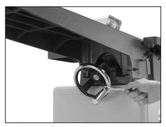
Figure 16. Securing the handwheel handle.
